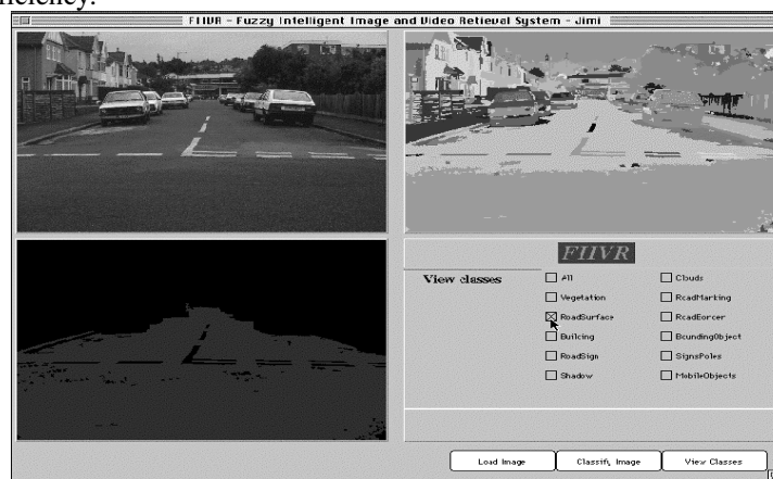
Figure 5: (top left) The original image, (top right quadrant) k-means segmented image and (bottom left quadrant) the results of region classification using in this case a rule-based ACGF model. The regions classified as road are highlighted in grey and the non-road regions are displayed in black.
