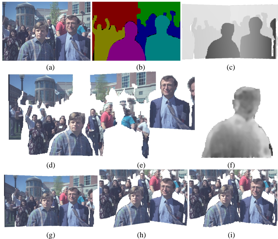
Figure 3: Layered stereo results: (a) third of five images; (b) initial segmentation into six layers; (c) recovered depth map (darker denotes closer); (d) and (e) the five layer sprites; (f) residual depth image for fifth layer. (g) re-synthesized third image (note extended field of view). (h) novel view without residual depth; (i) novel view with residual depth (note the “rounding” of the people).
