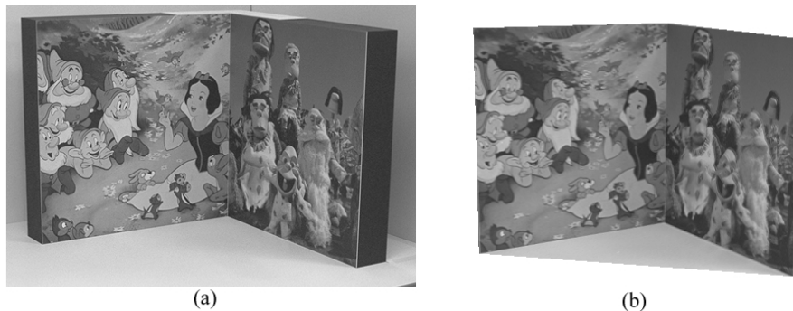
Figure 3: original and reconstruction of calibration targets
