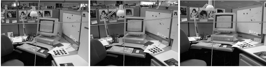
Figure 3: The trifocal junction point constraint. Figures (a) and (b) show straight lines fitted to a junction point. Figure (c) shows the lines projected into the third view.
