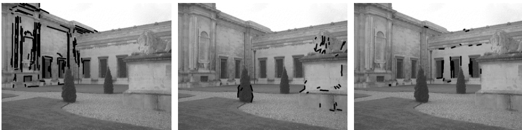
Figure 9: The following surfaces of the Fitzwilliam Museum, Cambridge, were found to be coplanar and are displayed using black lines.
