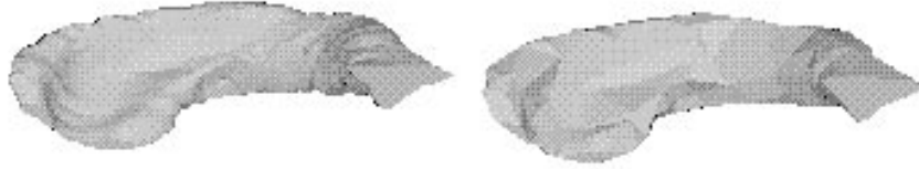
Figure 1: Result of applying the decimation algorithm to a triangulated surface of the left ventricle of the brain. On the left is a shaded representation of the original dense triangulation with approximately 2000 vertices. On the right the same surface represented by 200 vertices (decimated by 90%).
