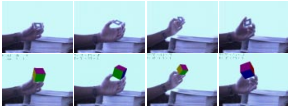
Figure 7: Frames in a video sequence are shown before and after augmentation with a virtual cube. The square pattern is the tracked target which is hidden by the virtual cube.
