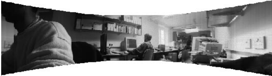
Figure 3: A planar mosaic made up of over 250 individual frames. The mosaic was created starting from the centre out to the right and then back upon itself to the left.
