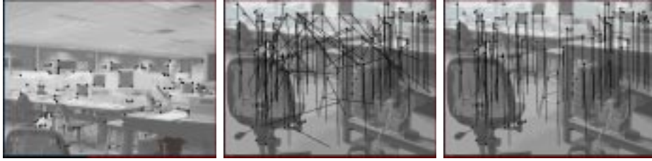
Figure 8: Example test results. The camera rotates about a horizontal axis between the two frames, resulting in a vertical image motion. Left: Image 1 with 110 corners overlaid. Centre: Image 2 with matches from the sum of squared differences matcher (3) with no threshold (this finds 97% of possible matches, with 35% outliers). Right: After filtering we are left with the same number of inliers, but only 4% outliers.
