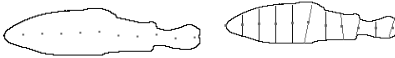
Figure 3: Illustration of length/width estimation: (a) initial skeleton points (column midpoints), (b) normal sections and final skeleton points.
