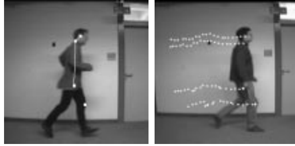
Figure 4: Left: Reference locations for the head (ear), trunk (neck) and leg (hip). The distances are marked. The fourth point is the knee, which is determined by the rotation of the leg and the length. Right: Trajectories of these four points out of 21 frames of a sequence.
