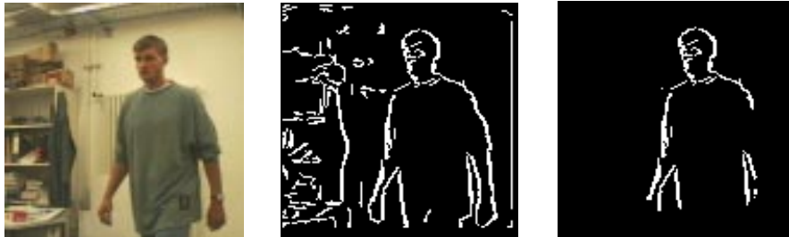
Figure 11: Person detection and model extraction using the combined method
