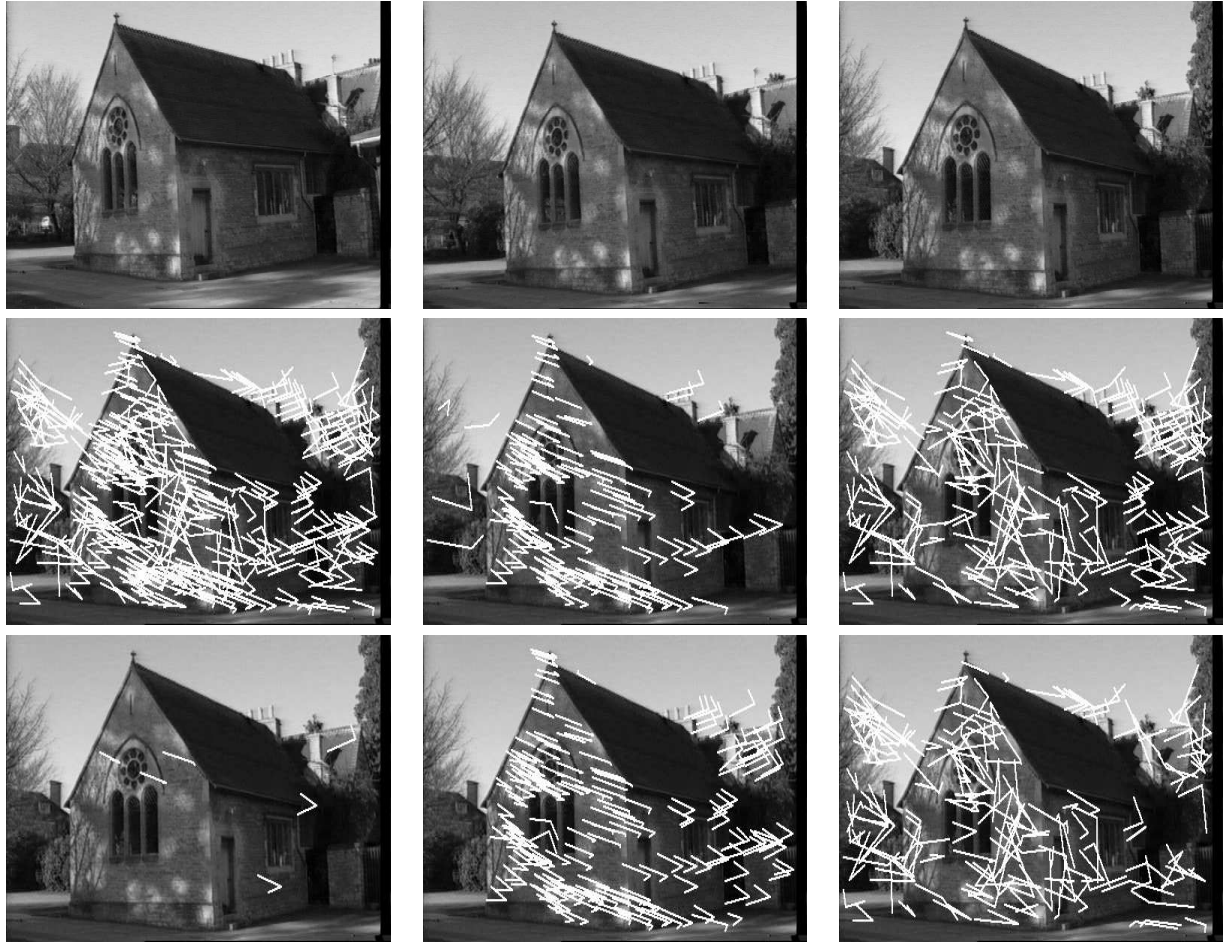
Figure 1: Top 3 images Three images from a sequence of a chapel, acquired by a hand-held camcorder. Camera motion is lateral and a few centimetres between frames. The image size is 760 \times 550 pixels. There are 341 corners tracked over all three images (from about 500 tracked pairwise). Middle 3 images Matches are shown for all three images, with the end points joined together and superimposed on the third image. The first shows all the matches, the middle shows the inliers after RANSAC and the right outliers. There are 146 inliers. After RANSAC the r.m.s. error between transferred points (using the trifocal tensor) and actual points in the third image is 2.5 pixels. Bottom 3 images Showing the results after the non-linear minimization. The left shows the six point basis selected by RANSAC. The middle shows the inliers after the non linear scheme, the right outliers. After the non-linear scheme the number of inliers has increased to 184. The r.m.s. error has decreased to 1.6 pixels. Note all the outliers on the tree to the left have been removed.
