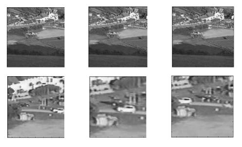
Figure 1: A three frame clip from an image sequence of over 90 frames. The top three images show a vehicle leaving the car park moving up a slight gradient in a left to right direction, at the same time a second vehicle is turning right and entering the car park. The car leaving the car park eventually occludes the vehicle that entered the car park. The lower three images show the corresponding enlarged portions of the original image where these vehicle are moving.
