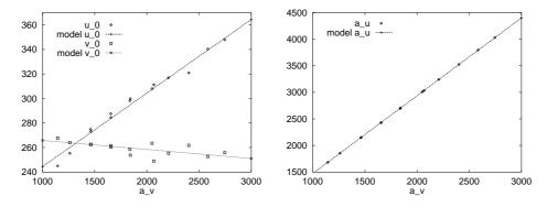
Figure 4: (a) Coordinates of the principal point  $(u_0, v_0)$  with respect to  $\alpha_v$ . (b)  $\alpha_u$  with respect to  $\alpha_v$ . The points in these graphs were obtained by classical calibration using a calibration grid ([11]). For each zoom position, several positions of the grid were used. The plotted lines represent the models found for the parameters' interdependence.
