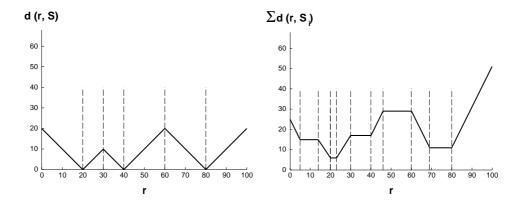
Figure 2: (a) d(r, S) for  $S = \{20, 40, 80\}$ . (b)  $d(r, S_1) + d(r, S_2)$  for  $S_1 = \{20, 40, 80\}$  and  $S_2 = \{5, 23, 69\}$ . The dotted lines indicate the abscissa where the functions have to be evaluated to find the global minimum.
