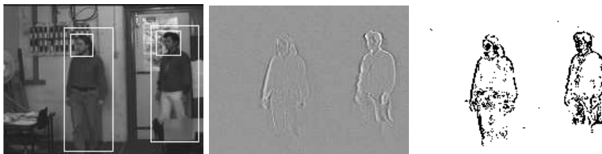
Figure 1: Motion-based tracking. Left: bounding boxes for tracked people and their heads. Centre: temporal convolution. Right: temporal zero-crossings.
