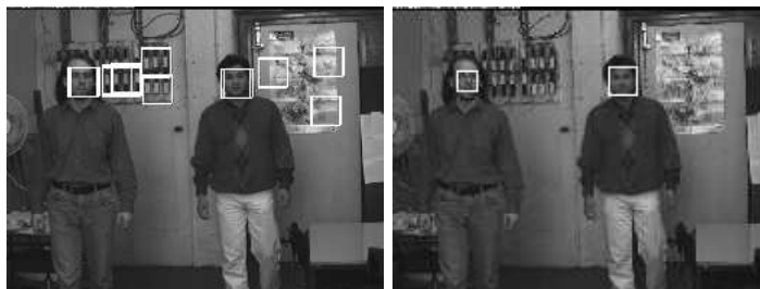
Figure 3: Left: Example output from a static face detector at a given scale. Erroneous detections occur due to “face-like” patterns. Right: Output when the motion-based tracker and the model-based face detector are combined.
