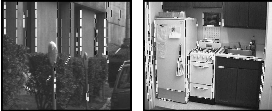
Figure 2: Images of a parking lot and kitchen scene from the VASC database. The detected line segments have been superimposed on the images. Long lines in the images have been detected as series of short line segments because the line detector has been applied to a series of 40 \times 40 pixel windows to duplicate the effect of real time processing. Section 3 explains how the entire extent of the line is recovered during tracking.
