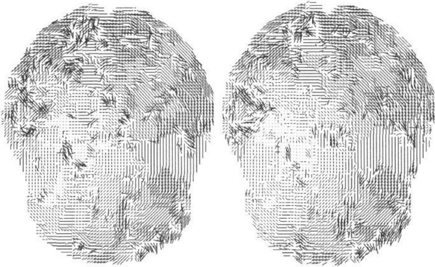
Figure 2: Mapping vectors between the initial and later images (left) using T2 correlation only and (right) using both T2 and PD data. A perfect match output should show all vectors “swirling” about a point just left of the centre of the brain. A mis-mapping is observable as a cross-hatching of overlapping vectors, whereas good mappings are largely all parallel.
