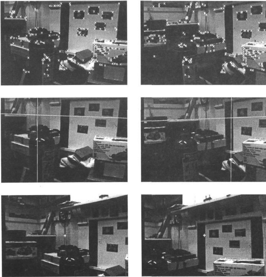
Figure 4: Left and right stereo pairs of the lab scene showing, from top to bottom: the final pair of images with corners superimposed (matched in white, unmatched in black); the computed lines at infinity in left and right views; the images after camera alignment with the image centres indicated by a cross-hair.
