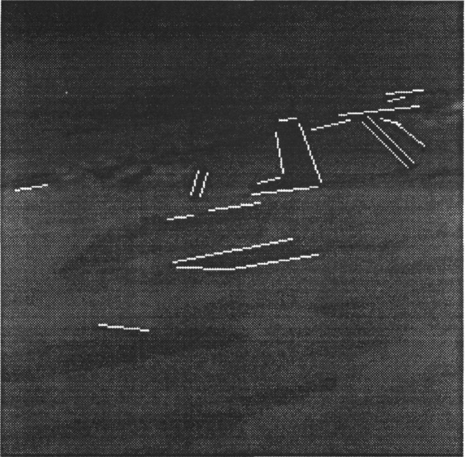
Fig 3: Runway seen from an approaching aircraft. Vanishing point is determined from the sides of the runway.
