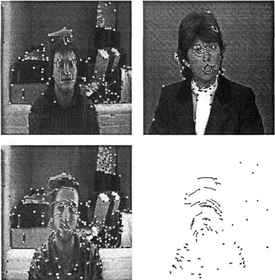
Figure 4: Image trajectories, each spanning an equal number of frames (true-length vectors, markers show corner positions in final frame): [top to bottom, left to right] “Richard” (8 frames); “Clair” (6 frames); “Dave” (6 frames); moving points for “Dave”.
