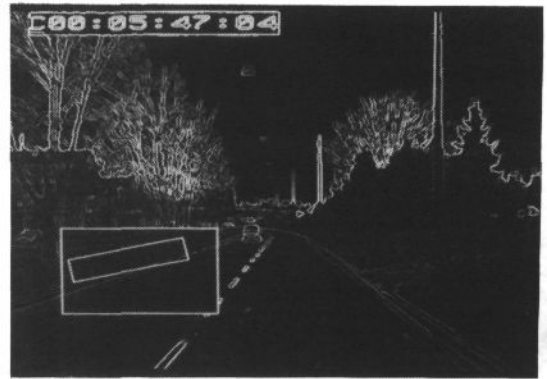
Figure 5. Approximation of the left road side by the RI which is calculated out of all CP in window 1 with gradient directions 66 \pm 16 deg. (see Fig. 3).
