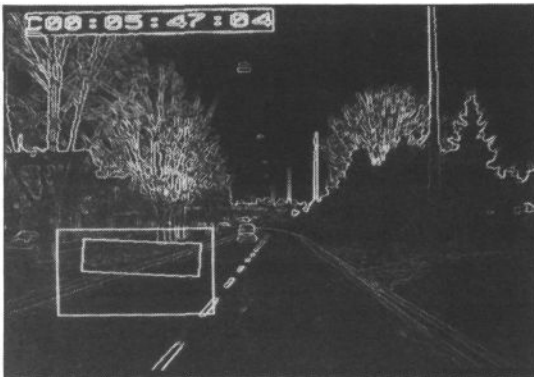
Figure 4. The gradient magnitude of all CP of Fig. 2 above the threshold 10 for a gradient operator with \sigma = 1.0 . In window 1 the RI (rectangle of Inertia) of these CP (see text) is shown.
