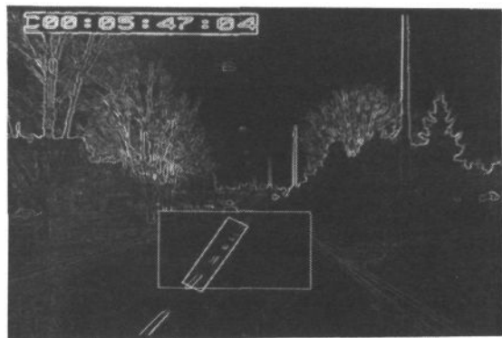
Figure 10. The RI in window 2 corresponds to a MST subtree which contains 90 % of the CP with gradient directions 24 \pm 16 and 210 \pm 16 deg.
