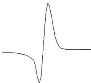
Figure 11: Cross-section of wave/diffusion displacement – the wave is travelling from left to right.
