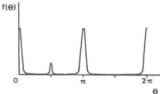
Figure 7 Distribution of boundary orientations for the comb shape
