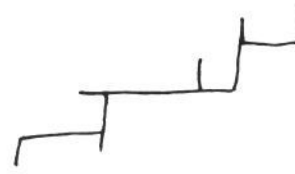
Figure 5. When zero-crossings are taken individually for differences in different directions, a boundary may have "feathering," i.e. short extra boundary markings off to each side.
