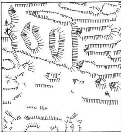
c) Enlargement of portion of b) to show individual edge and motion fragments. Stems of T's indicate magnitude of motion orthogonal to local edge fragments.
