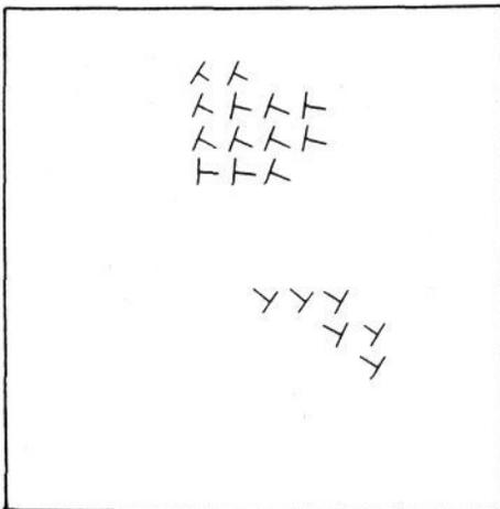
b) Flow vector map from 32 x 32 pixel progressive window analysis with rejection of vectors where local 3 x 3 patch has orientation uncertainty greater than 20 degrees.
