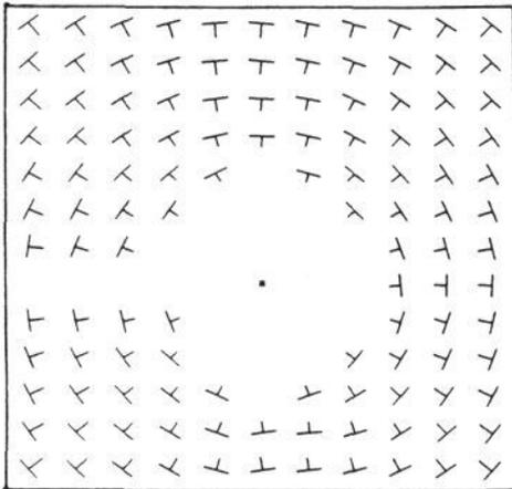
b) Motion vector map from a 64 x 64 pixel window analysis. Motion vectors having a local 3 x 3 orientation uncertainty of greater than 20 degrees are suppressed. The computed focus of expansion is shown by the spot in the central region of the vector map.
