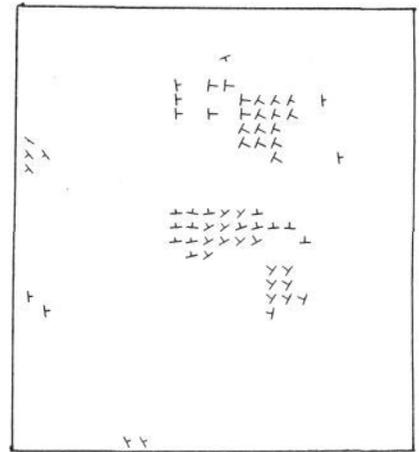
e) As d), but with rejection of vectors where local 3 x 3 patch has orientation uncertainty greater than 20 degrees.
