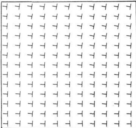
c) Motion vector map from a 64 x 64 pixel window analysis for a situation where the sensor was approaching the village scene of figure 5a with additional large translational motion in X.
