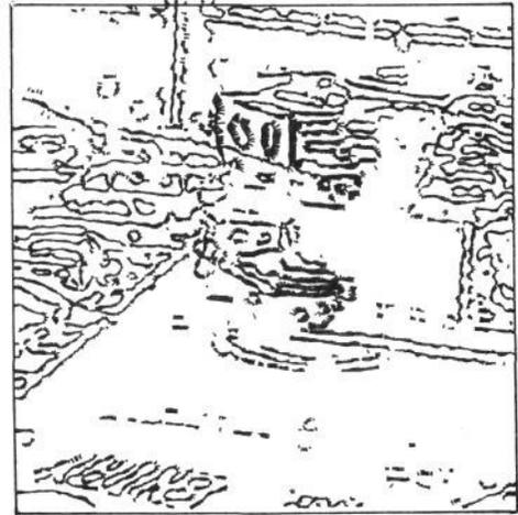
b) Fragmentary edge and motion output from paired-frame analysis. "Thickening" of profiles indicates local flow magnitude.
