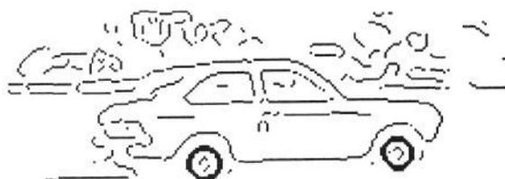
**Figure 3.** Analysis of edges present in the larger boxed region of Figure 2. Each connected edge is labelled by its curvature and type (line, arc, closed curve). Acceptable wheel instances are emphasised.
