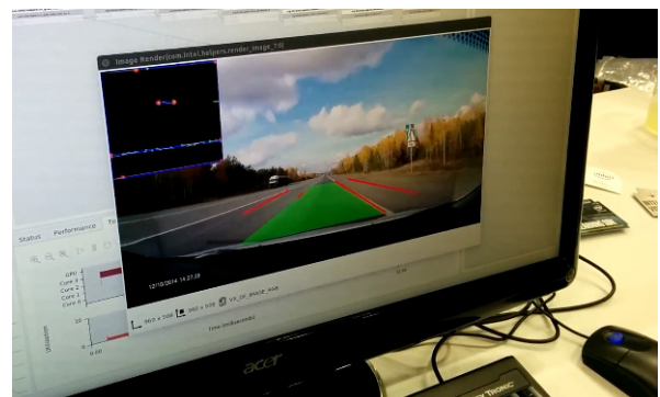
An Intel tech demo of real-time lane detection algorithm that was rapidly created using OpenVX
